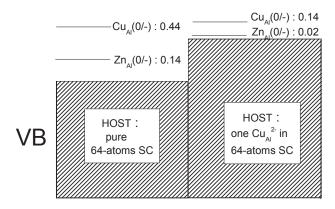
Fig. 3. Calculated acceptor defect levels  $\varepsilon(0/-)$  of  $Cu_{Al}$  and  $Zn_{Al}$  based on two different hosts [i.e., pure  $CuAlS_2$  and one  $Cu_{Al}^{2-}$  existing in a 64-atom  $CuAlS_2$  supercell (SC)].
