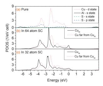
Fig. 1. Partial densities of states (PDOSs) of Cu-3d, Al-3s, and S-3p,4s in  $CuAlS_2$  (a) and the PDOSs of Cu-3d of the  $Cu_{Al}^0$  defect and Cu atom in one  $Cu_{Al}^0$  in  $CuAlS_2$  64-atom (b) and 32-atom (c) supercells.
