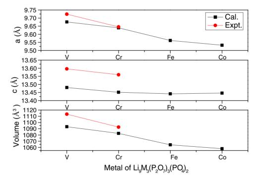
Figure 2. Calculated crystal parameters and voltages of  $\text{Li}_9M_3(\text{P}_2\text{O}_7)_3(\text{PO}_4)_2$  (M = Fe, Cr, Co, V), with experimental values [16, 19] displayed in red.
