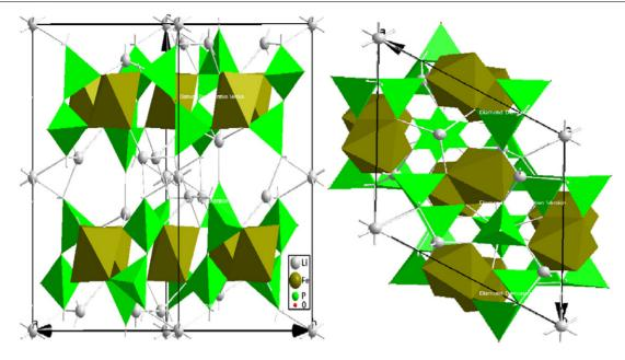
Figure 1. Structure of  $\text{Li}_9M_3(\text{P}_2\text{O}_7)_3(\text{PO}_4)_2$  (M = V, Fe, Cr, Co).
