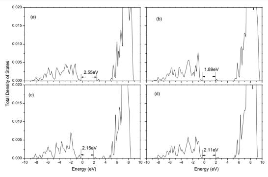
**Figure 3.** Total density of states for  $\text{Li}_9M_3(\text{P}_2\text{O}_7)_3(\text{PO}_4)_2$ . (a)  $\text{Li}_9\text{Cr}_3(\text{P}_2\text{O}_7)_3(\text{PO}_4)_2$  with U=3.5; (b)  $\text{Li}_9\text{Co}_3(\text{P}_2\text{O}_7)_3(\text{PO}_4)_2$  with U=5.0; (c)  $\text{Li}_9\text{V}_3(\text{P}_2\text{O}_7)_3(\text{PO}_4)_2$  with U=4.0; (d)  $\text{Li}_9\text{Fe}_3(\text{P}_2\text{O}_7)_3(\text{PO}_4)_2$  with U=4.5.
