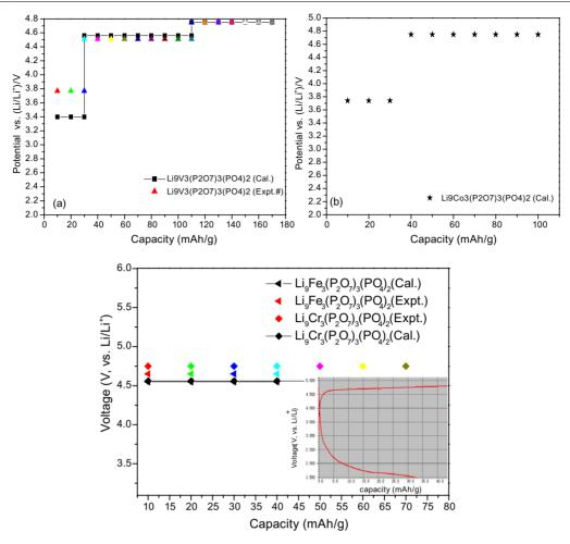
**Figure 4.** The charge and discharge profile of  $\text{Li}_9M_3(\text{P}_2\text{O}_7)_3(\text{PO}_4)_2$  (M = V, Fe, Co and Cr) by first-principles calculation, along with the experimental values [16–19]. The charge and discharge curve of  $\text{Li}_9\text{Fe}_3(\text{P}_2\text{O}_7)_3(\text{PO}_4)_2$  is shown in the insert figure of figure 6(c) [22].
