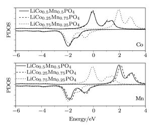
**Fig. 5.** The PDOS of Co and Mn atoms in  $\text{LiCo}_{1-x}\text{Mn}_x\text{PO}_4/\text{Co}_{1-x}\text{Mn}_x\text{PO}_4$  for  $x=0.25,\ 0.5$  and 0.75.
