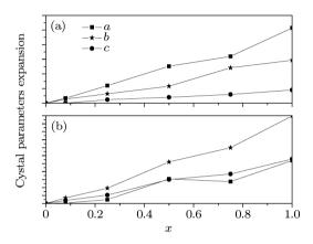
**Fig. 2.** Crystal parameter expansion of Mn doped structure with different x for (a)  $\text{LiCo}_{1-x}\text{Mn}_x\text{PO}_4$  and (b)  $\text{Co}_{1-x}\text{Mn}_x\text{PO}_4$ .
