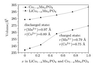
**Fig. 3.** Volume change of  $\text{LiCo}_{1-x}\text{Mn}_x\text{PO}_4$  and  $\text{Co}_{1-x}\text{Mn}_x\text{PO}_4$  with different x values.
