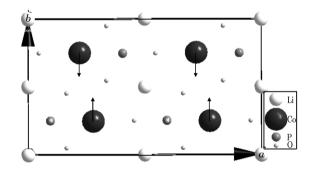
Fig. 1. The stable AFM spin configuration of  $LiCoPO_4$ .
