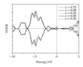
**Fig. 4.** Total density of states of  $\text{LiCo}_{1-x}\text{Mn}_x\text{PO}_4$ ; the Fermi level is set as a reference.
