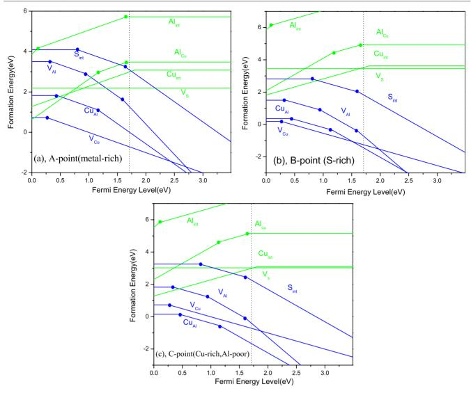
**Figure 3.** The formation enthalpy of intrinsic defects in  $CuAlS_2$  under different conditions with the potential alignment and image charge correction. Red and blue lines represent the donor and acceptor defects, respectively. Here the experimental gap of  $CuAlS_2$ ,  $E_g = 3.49 \, eV$ , is adopted. (Colour online.)
