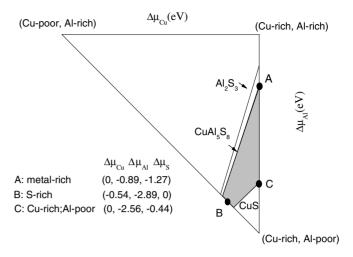
**Figure 2.** The chemical potential ranges for a stable CuAlS<sub>2</sub>. The grey areas are the allowed chemical potential range for CuAlS<sub>2</sub> with consideration of competing compounds. Points A, B and C represent three extreme conditions considered in this work.
