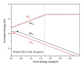
**Figure 5.** The formation enthalpies of Mg ( $\Delta\mu_{\text{Mg}}=-2.53\,\text{eV}$ ) and Zn ( $\Delta\mu_{\text{Zn}}=-1.23\,\text{eV}$ ) doped in CuAlS $_2$  under Cu-rich and Al-poor condition (point C in figure 4). Solid lines and dashed lines represent the acceptor and donor defects, respectively. Here the experimental gap of CuAlS $_2$ ,  $E_g=3.49\,\text{eV}$ , is adopted. (Colour online.)
